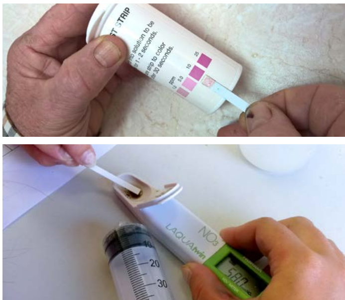
Figure 13. Nitrate strip test and LAQUAtwin nitrate sensor
