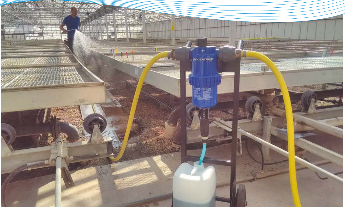
Figure 1. Proportional dilutors are essential items of nursery equipment permitting the delivery of soluble fertilisers, entomopathogenic nematodes, plant protection products and other liquid concentrates
